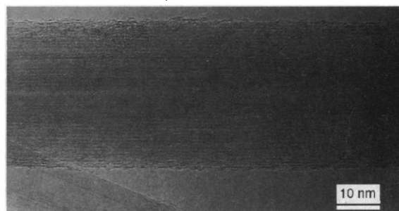
Fig. 3. High-resolution TEM image of a carbon nanotube. The tube is well graphitized and consists of about 40 concentric shells of carbon sheets with spacing between the sheets of 0.34 nm. The inner and outer diameters of the tube are 4 and 34 nm, respectively. Several TEM specimens have been examined carefully, but no carbon nanoparticles or iron nanoparticles trapped inside the tubes were observed, indicating that the carbon nanotube arrays are very pure.
