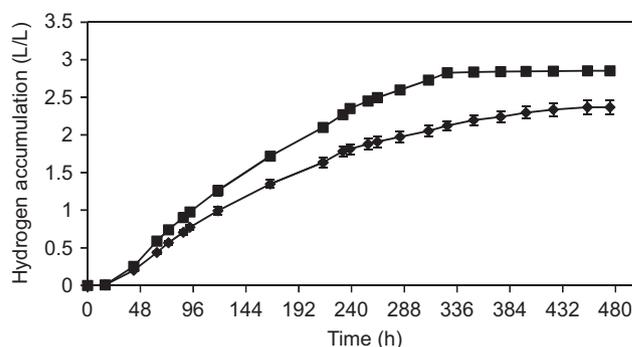
**Fig. 4 – Total hydrogen production by wild type (◆) and *hup*<sup>-</sup> mutant (■) *R. sphaeroides* O.U.001. Each value in the curves is the mean of three times replication with  $\pm$  standard deviation.**
