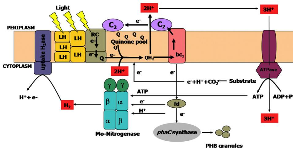
Fig. 1 – The schematic view of  $H_2$  related pathways in *R. sphaeroides*.
